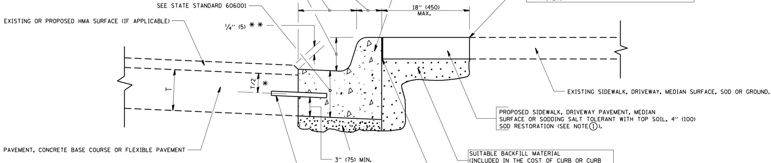
\* 3" (75) MINIMUM FROM TOP AND BOTTOM OF THE CONCRETE PAVEMENT OR BASE COURSE.
