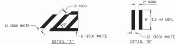
TYPICAL CROSSWALK MARKING
