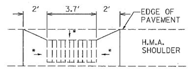
\* SLOPE TO MATCH EXIST. GRATE WHEN PLACING H.M.A. SHOULDERS.
