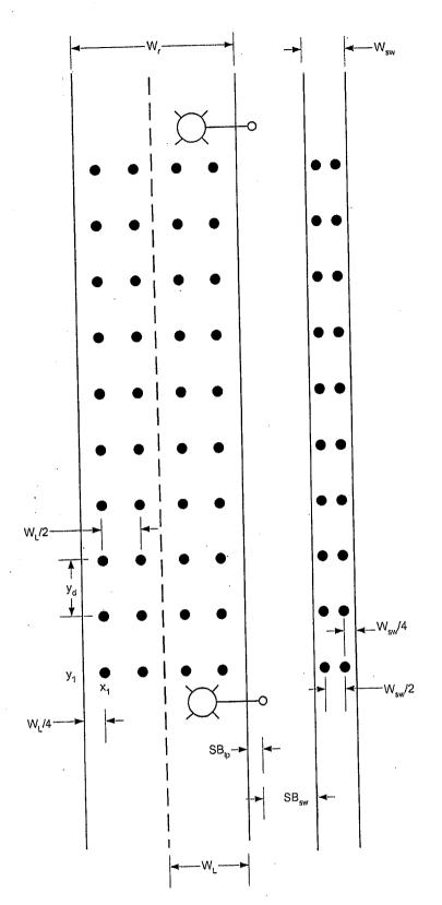
W<sub>r</sub> = Roadway Width W<sub>L</sub> = Lane Width W<sub>SW</sub> = Sidewalk Width SB<sub>LP</sub> = Light Pole Set Back SB<sub>SW</sub> = Sidewalk Set Back
