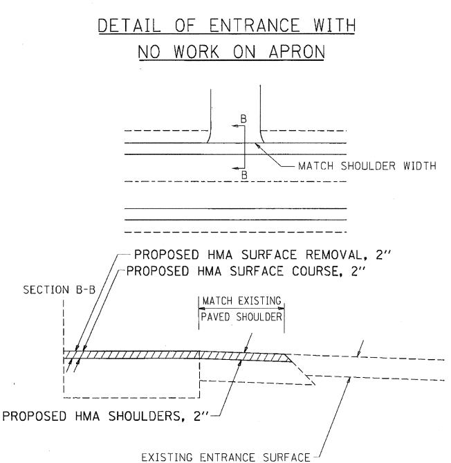
PREPARATION OF EXISTING SURFACE AND ANY EXCAVATION FOR ENTRANCES SHALL BE IN ACCORDANCE WITH ARTICLE 406.09 OF THE STANDARD OF SPECIFICATIONS.
