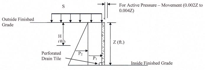
Figure 1, Earth Pressure Schematic
