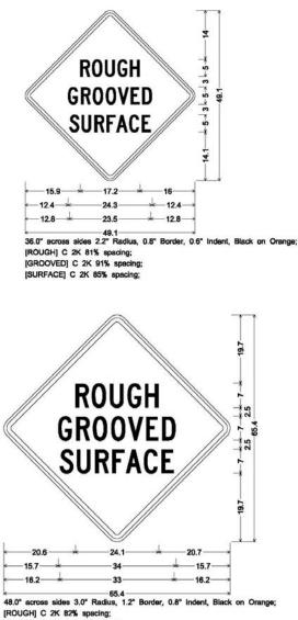
[GROOVED] C 2K 90% spacing; [SURFACE] C 2K 87% spacing;
