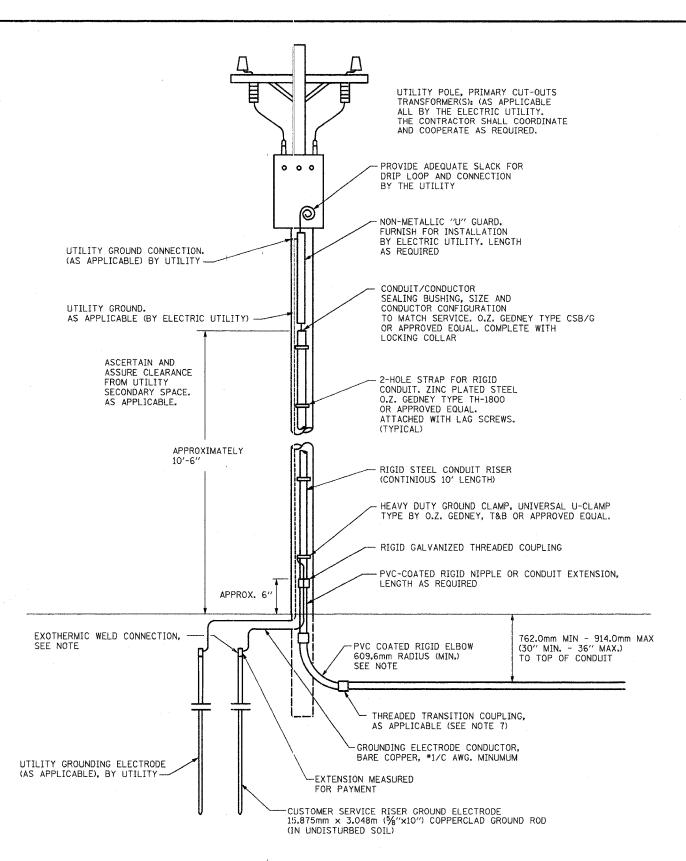
PROPOSED SERVICE INSTALLATION POLE TOP MOUNTED TRANSFORMER
