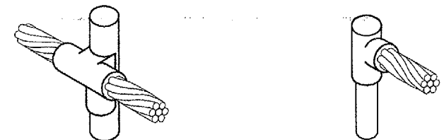
CABLE TO GROUND ROD
