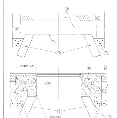
BRICK, MORTAR, OR CONC. ADJUSTING RINGS
