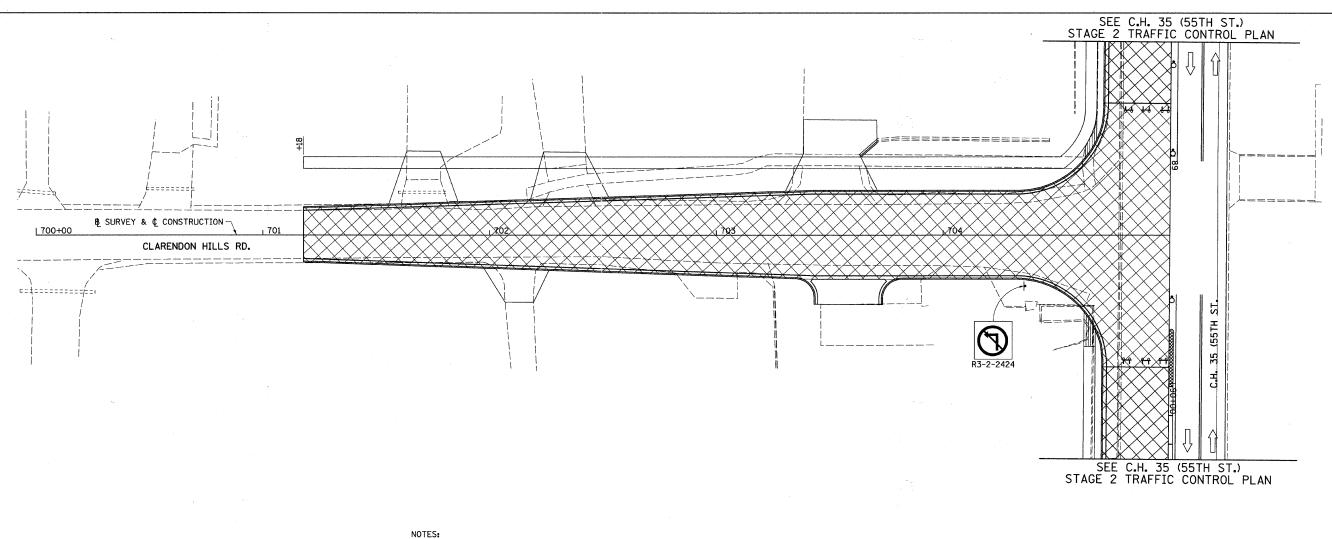
SEE TRAFFIC CONTROL AND STAGING PLAN FOR TRAFFIC CONTROL AND PROTECTION, MAINTENANCE OF TRAFFIC AND STAGE CONSTRUCTION NOTES. EAST SIDE TO BE CONSTRUCTED FIRST, THEN THE WEST SIDE.
