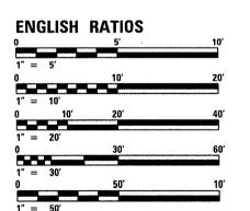
PLANS HAVE BEEN PREPARED USING STANDARD ENGINEERING SCALES. REPRODUCED PLANS WILL NOT CONFORM TO STANDARD SCALES. IN MAKING MEASUREMENTS ON REPRODUCED PLANS, THE ABOVE SCALES MAY BE USED.
