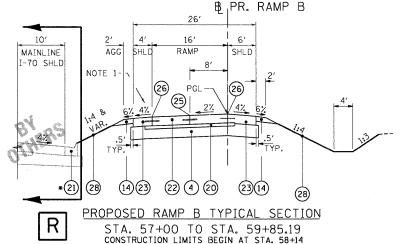
SHOULDER TRANSITIONS FROM 2% (57+00) AT ANCHORAGE SLAB TO 4% (57+25).
