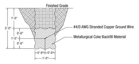
Figure 5. Grounding Trench Detail
