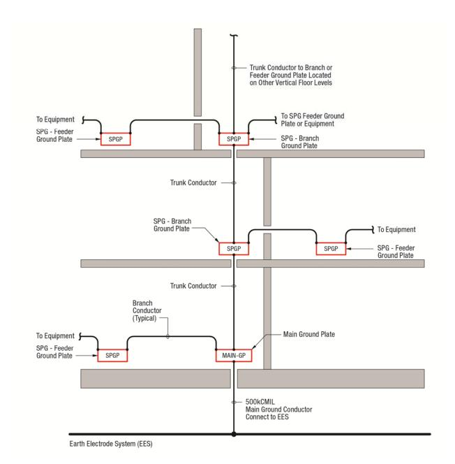
Figure 20. Single-Point Ground System Installation – Illustrative Example
