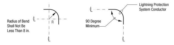
CONDUCTOR BENDING REQUIREMENTS
