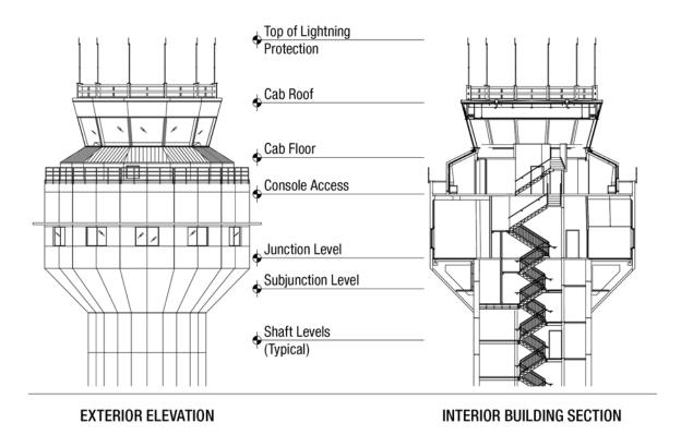
Figure 14. Airport Traffic Control Tower – Typical Floor Levels
