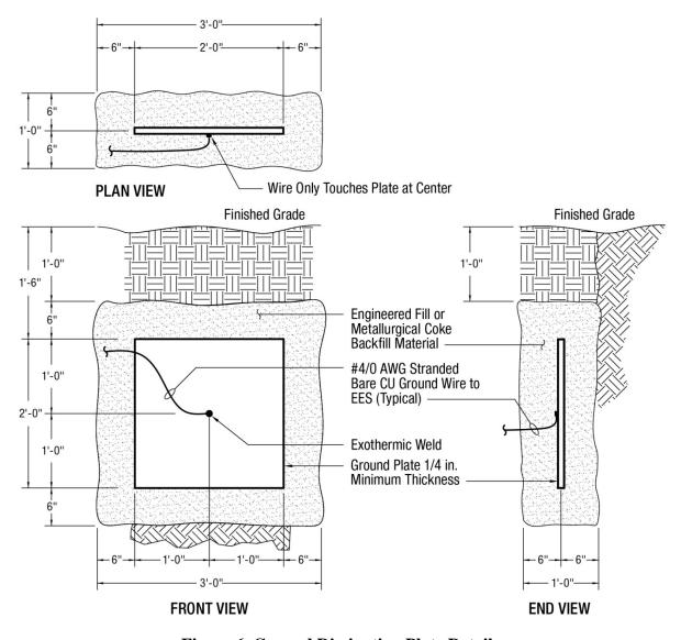
Figure 6. Ground Dissipation Plate Detail
