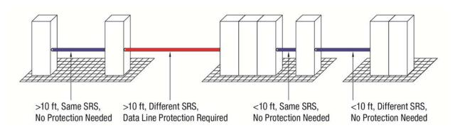
Figure 21. Lines and Cables Requiring Protection
