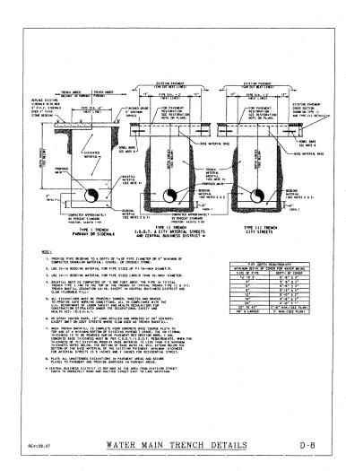
5) FITTINGS AND THEIR LOCATIONS INDICATED ON THE DRAWINGS ARE TENTATIVE. THE CONTRACTOR MUST COMPLETE THE INSTALLATION WITH THE NECESSARY FITTINGS DICTATED BY FIELD CONDITIONS. NO ADDITIONAL PAYMENT WILL BE MADE FOR DEVIATIONS FROM THE INDICATED FITTINGS.
