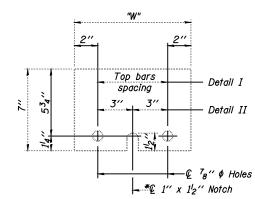
STEEL RETAINER P 1" x 7" x 10" \* Required only with Detail II
