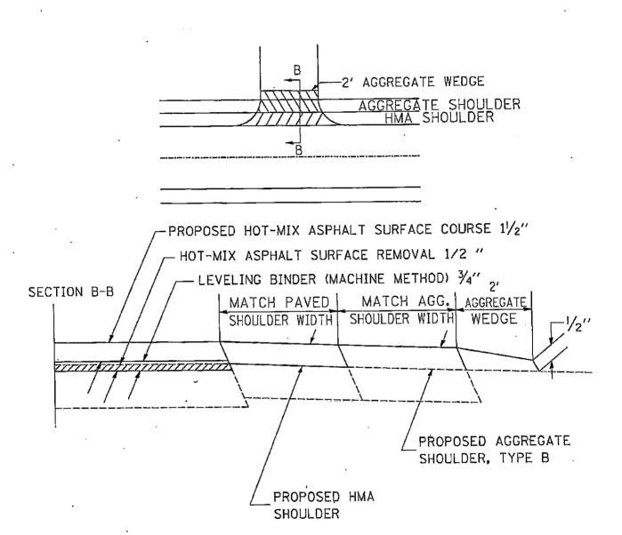
PREPARATION OF EXISTING SURFACE AND ANY EXCAVATION FOR ENTRANCES SHALL BE IN ACCORDANCE WITH ARTICLE 406.09 OF THE STANDARD SPECIFICATIONS.
