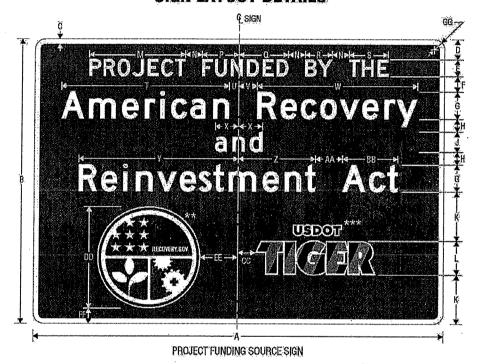
NOTE: SIGN SHALL NOT BE INSTALLED WITHOUT PROJECT FUNDING SOURCE PLAQUE
