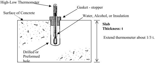
Scheme for measuring concrete temperature below the surface.
