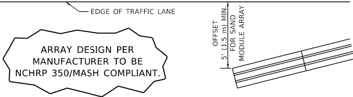
DETAIL "A" IMPACT ATTENUATOR, TEMPORARY (SEE NOTE 5)
