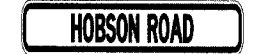
③③ R TYPE (SPECIALTY) 48" X 6" PANEL 3" D BLACK LETTERS WHITE BACKGROUND BLACK BORDER
