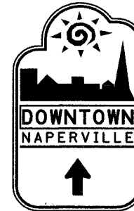
②⑤ SPECIALTY SIGN 30" X 48" PANEL WHITE AND BROWN LETTERS WHITE BACKGROUND BROWN BORDER
