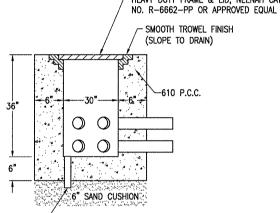
2" SCHED 40 PVC DRAIN PIPE. NOTE 6" OF CA-7 GRAVEL MAY BE PROVIDED, INSTEAD OF 6" CONCRETE FLOOR WITH DRAIN PIPE, AT CONTRACTORS OPTION.
