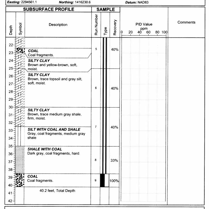
Note 1: Backfilled hole with bentonite slurry grout 0-40.2'.
