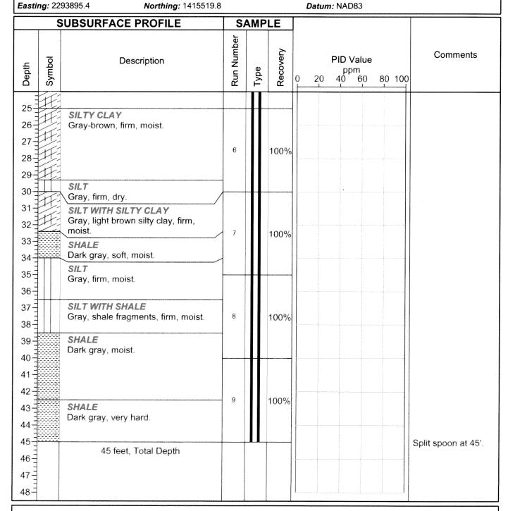
Note 1: Backfilled hole with bentonite slurry grout 0-45'.
