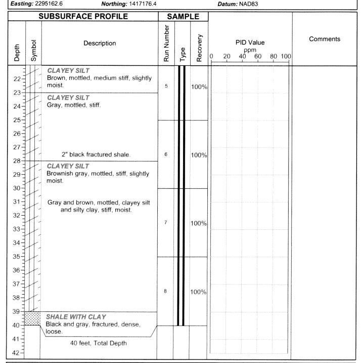
Note 1: Backfilled hole with bentonite slurry grout 0-40'.
