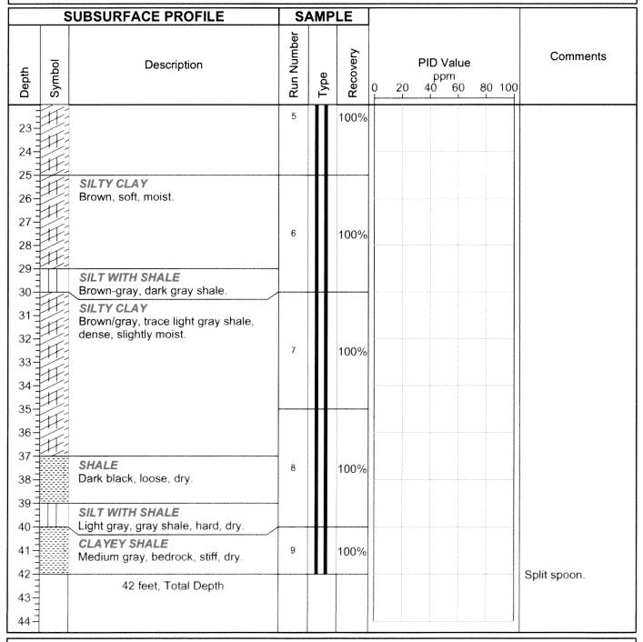
Note 1: Backfilled hole with bentonite slurry grout 0-42'.
