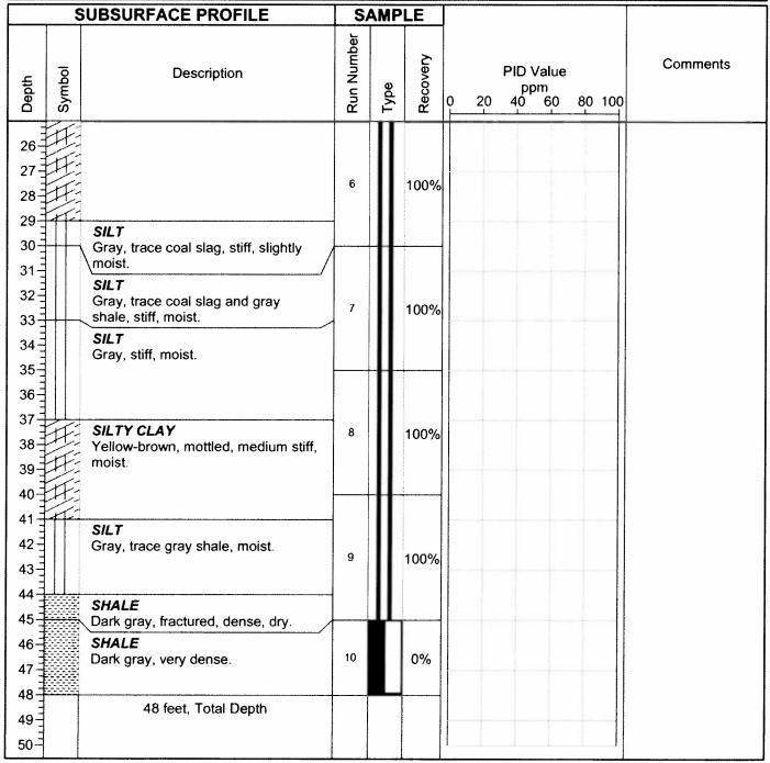
Note 1: Backfilled hole with bentonite slurry grout 0-48'.
