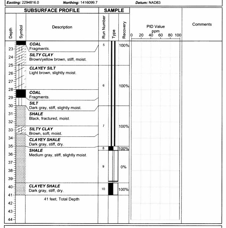
Note 1: Backfilled hole with bentonite slurry grout 0-41'.
