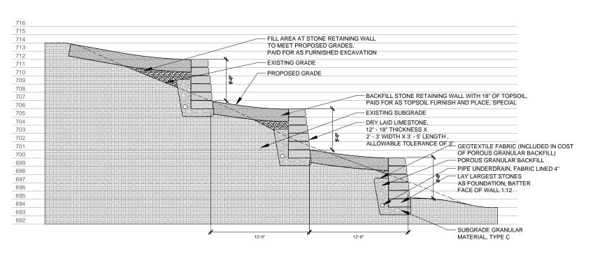
NOTE: SECTION IS TYPICAL, SPECIFIC CONDITIONS WILL VARY BASED ON STONE RETAINING WALL CONFIGURATION AND GRADES INDICATED ON GRADING PLAN.
