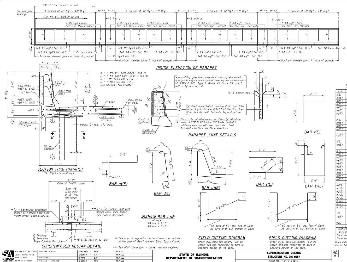
Notes: Reinforcement bars shall not pass thru aluminum sheets and cork joint filler. All dimensions are along front face of parapet.
