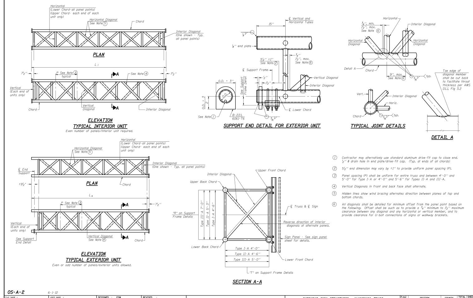
USER NAME = DESIGNED - ESW REVISED SECTION COUNTY OVERHEAD SIGN STRUCTURES - ALUMINUM TRUSS STATE OF ILLINOIS CHECKED JWS REVISED 57/70 (25-4)R EFFINGHAM 1760 410 DETAILS FOR TRUSS TYPES I-A, II-A AND III-A PLOT SCALE = DRAWN PDB REVISED **DEPARTMENT OF TRANSPORTATION** CONTRACT NO. 74295 SHEET NO. 23 OF 53 SHEETS PLOT DATE = CHECKED REVISED BRM
