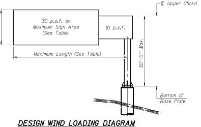
Parameters shown are basis for I.D.O.T. Standards Installations not within dimensional limits shown require special analysis for all components.
