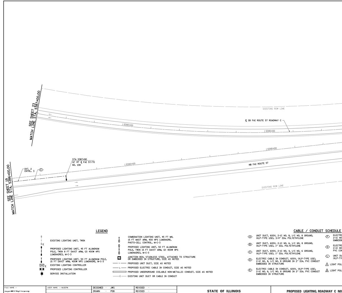
**PROPOSED LIGHTING, ROADWAY** PLOT SCALE = \$SCALE\$ CHECKED BRM REVISED **DEPARTMENT OF TRANSPORTATION** SCALE: 1"=50' SHEET NO. 20 OF 35 SHEETS PLOT DATE = \$DATE\$ DATE 11-02-12 REVISED
