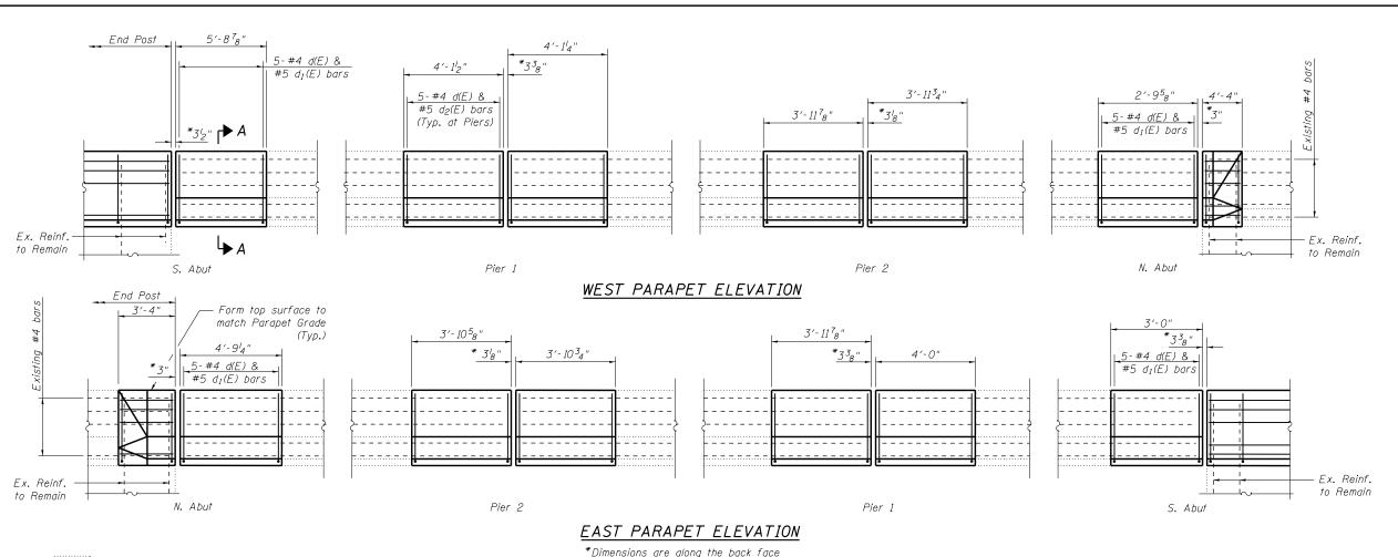
\*Dimensions are along the back face of the parapet at 50° F.
