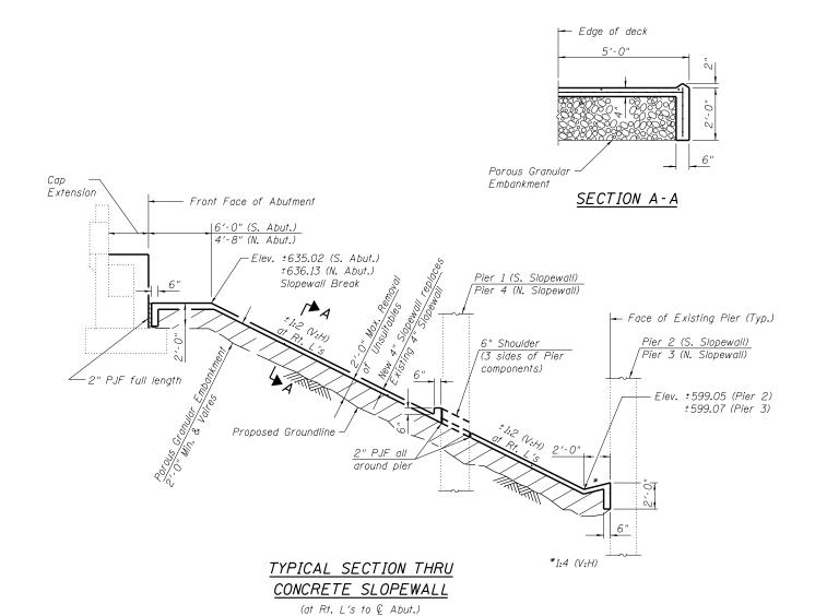
Indicates Removal of Unsuitable Materials and replacement with Porous Granular Embankment
