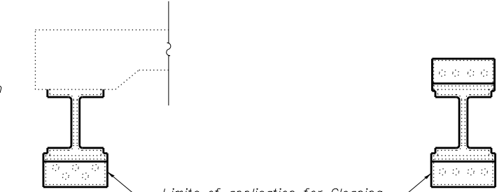
Limits of application for Cleaning and Painting Steel Bridge SECTION A-A SHOWING DIAPHRAGM D1 SHOWING DIAPHRAGM D2 SECTION B-B Limits of application for Cleaning and Painting Steel Beams (Typ.) SECTION C-C Limits of application for Cleaning and Painting Steel Bridge SECTION D-D
