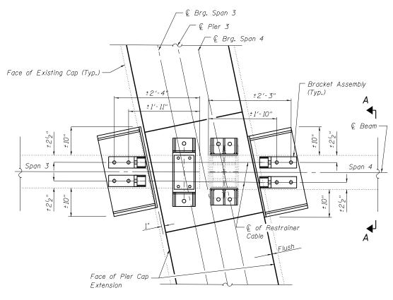
RESTRAINER INDICATOR END RESTRAINER BOLTED END
