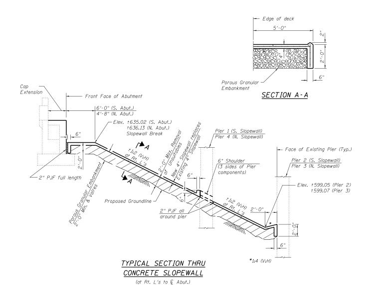
Indicates Removal of Unsuitable Materials and replacement with Porous Granular Embankment
