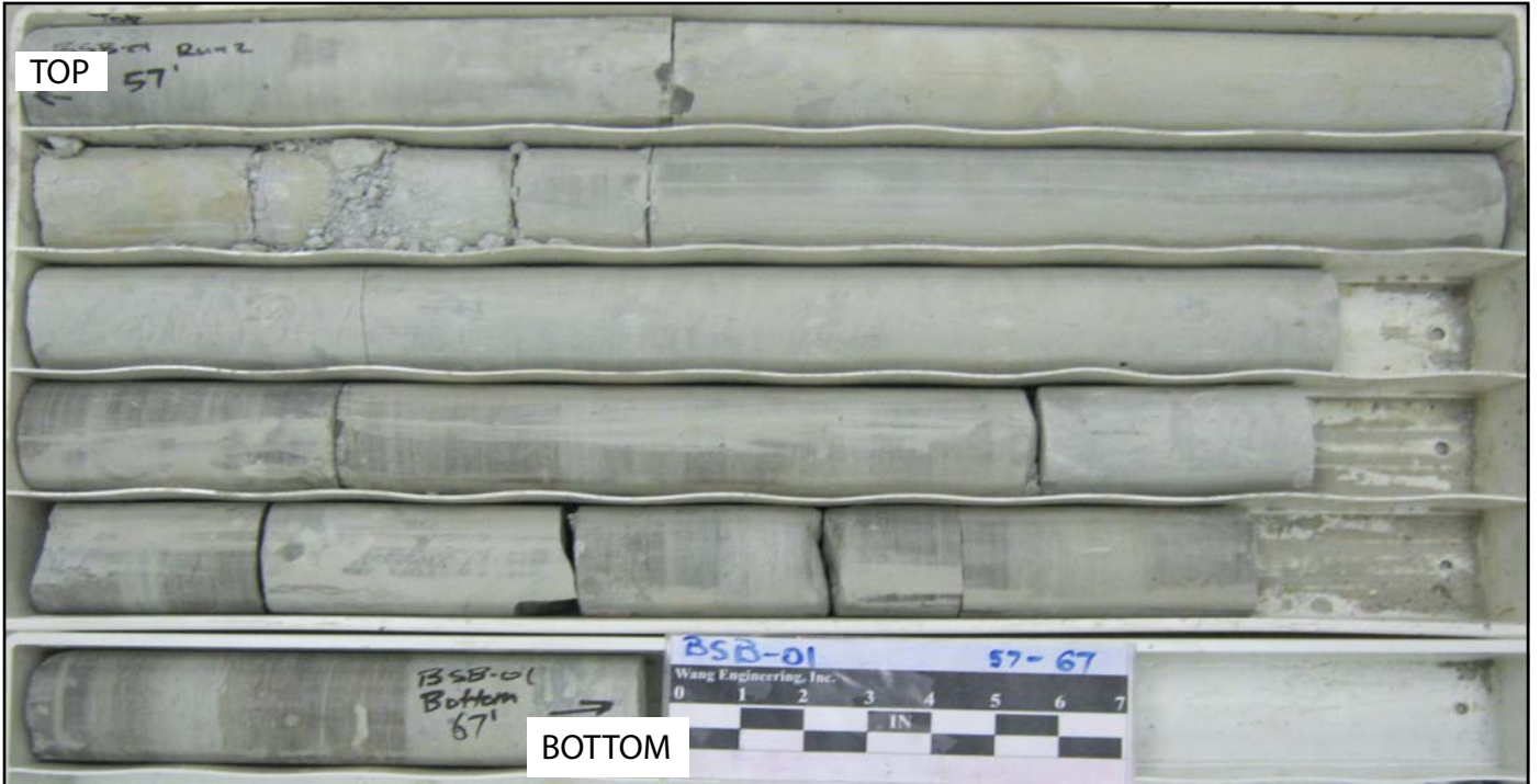
Boring BSB-01 Run #2, 57' to 67', RECOVERY=100%, RQD=88%
