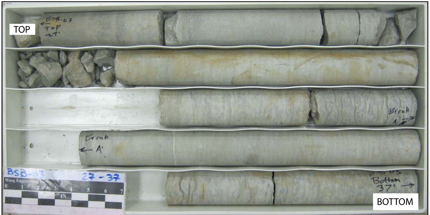
Boring BSB-03 Run #1, 27' to 37', RECOVERY=78%, RQD=63%
