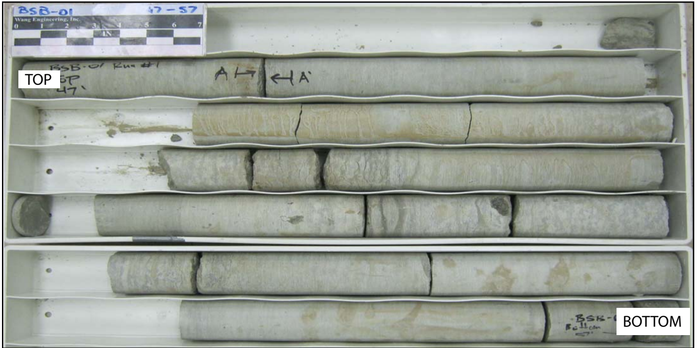
Boring BSB-01 Run #1, 47' to 57', RECOVERY=96%, RQD=85%
