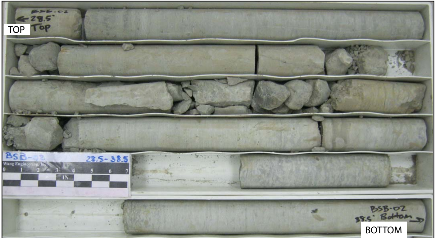
Boring BSB-02 Run #1, 28.5' to 38.5', RECOVERY=100%, RQD=68%
