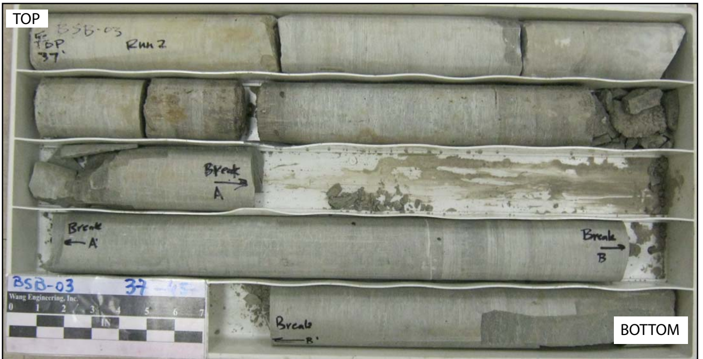
Boring BSB-03 Run #2, 37' to 45', RECOVERY=94%, RQD=88%
