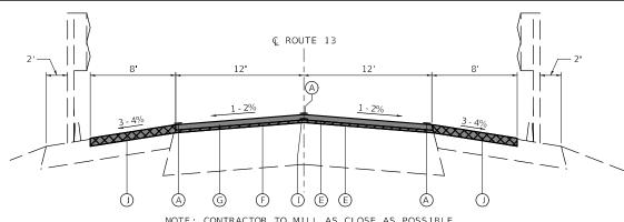
NOTE: CONTRACTOR TO MILL AS CLOSE AS POSSIBLE WITHOUT IMPACTING THE EXISTING GUARDRAIL.
