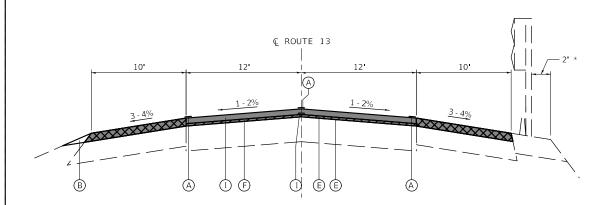
NOTE: CONTRACTOR TO MILL AS CLOSE AS POSSIBLE WITHOUT IMPACTING THE EXISTING GUARDRAIL.
