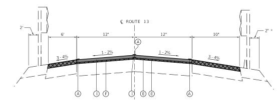
NOTE: CONTRACTOR TO MILL AS CLOSE AS POSSIBLE WITHOUT IMPACTING THE EXISTING GUARDRAIL.
