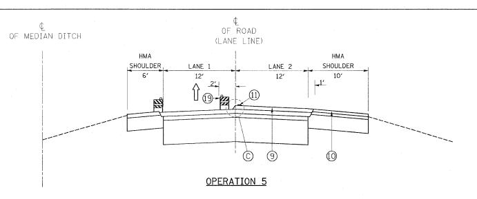
(9) RESURFACING WITH SMA SURFACE COURSE 2" ON LANE 2. (11) TEMPORARY PAVEMENT MARKING
