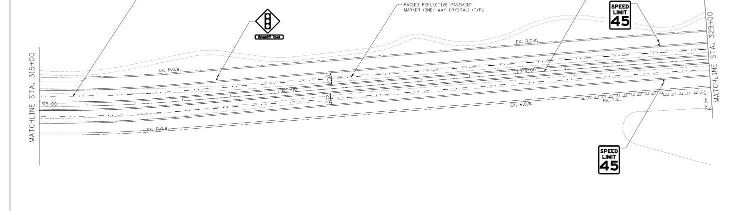
— POLYUREA PAVEMENT MARKING TYPE I - LINE 4" (SKIP - DASH WHITE, 30' SKIP - 10' DASH) (TYP.) —¢ U.S. ROUTE 30
