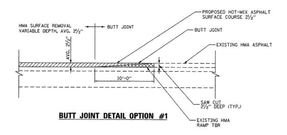
NOTE: RAMPING DOWN DURING HOT-MIX ASPHALT SURFACE REMOVAL, VARIABLE DEPTH WILL NOT BE PAID FOR AS TEMPORARY RAMP.
