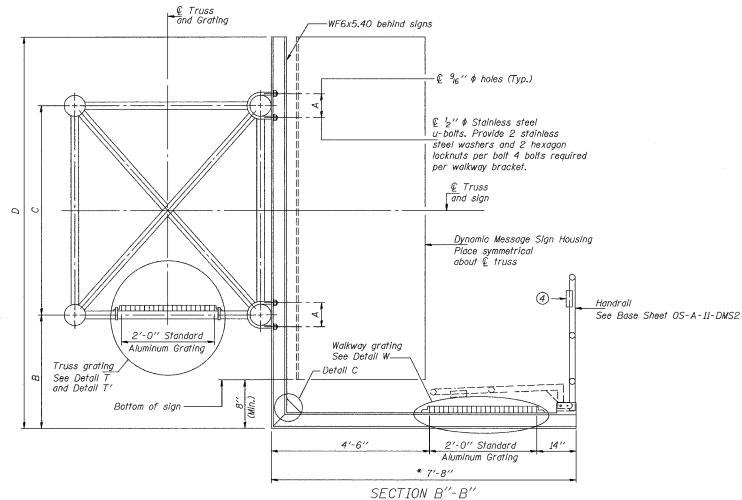
\* Bracket and grating dimensions are nominal and will vary based on actual DMS cabinet dimensions plus manufacturer's mounting devices, and providing clearance between the lowered handrall and DMS cabinet.
