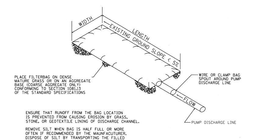
SILT INTO EXISTING TOPOGRAPHY, SEED AND MULCH MAINTAIN EXTRA FILTER BAGS ON SITE. REPLACE DAMAGED BAGS PROMPTLY.
