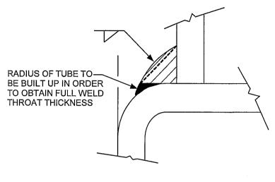
FIGURE 7.1 BUILD UP RADIUS WELD
