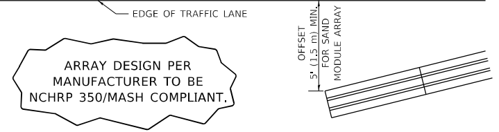
DETAIL "A" IMPACT ATTENUATOR, TEMPORARY (SEE NOTE 5)
