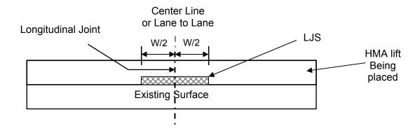
The width and minimum application rate shall be according to the following table:
