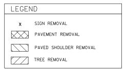
NOTE: TREE REMOVAL LAYOUT IS RELATIVE TO THE PROPOSED ALIGNMENT.
