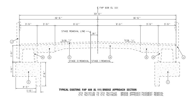
NOTE: BRIDGE APPROACH PAVEMENT REMOVAL SHALL BE PAID FOR AS "PAVEMENT REMOVAL".
