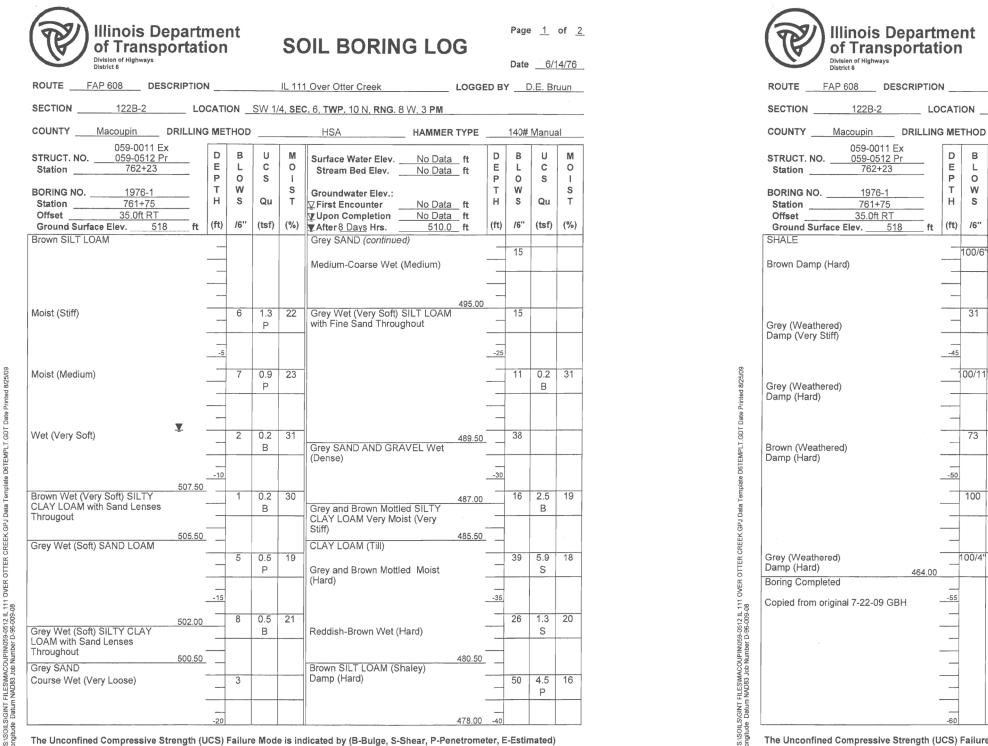
The Unconfined Compressive Strength (UCS) Failure Mode is indicate Abbreviations W.O.H - Sampler Advanced By Weight of Hammer, W.O. The SPT (N value) is the sum of the last two blow values in each same
