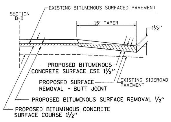
IF EXISTING BASE COURSE IS INADEQUATE, AS DETERMINED BY THE ENGINEER, THE SIDEROADS SHALL BE CORED OUT AND AGGREGATE BASE COURSE, TYPE B SHALL BE PLACED FOR BASE. THE COST OF CORING OUT THE SIDEROAD SHALL BE INCLUDED IN THE COST OF THE AGGREGATE BASE COURSE. IF EXISTING BASE COURSE IS DETERMINED TO BE ADEQUATE, THE AGGREGATE BASE COURSE SHALL BE DELETED AND THE PREPARATION OF THE BASE SHALL BE CONSTRUCTED ACCORDING TO ARTICLE 406.09.
