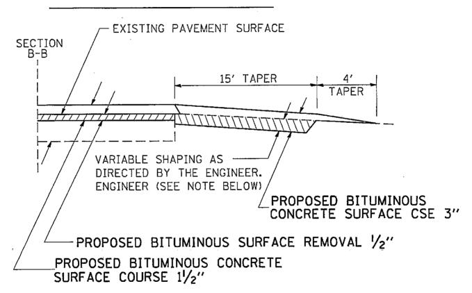
IF EXISTING SUB-BASE IS INADEQUATE, AS DETERMINED BY THE ENGINEER, THE SIDEROADS SHALL BE CORED OUT AND AGGREGATE SUB-BASE, TYPE B SHALL BE PLACED FOR BASE. THE COST OF CORING OUT THE SIDEROAD SHALL BE INCLUDED IN THE COST OF THE AGGREGATE BASE COURSE. IF EXISTING SUB-BASE IS DETERMINED TO BE ADEQUATE, THE AGGREGATE BASE COURSE SHALL BE DELETED AND THE PREPARATION OF THE BASE SHALL BE CONSTRUCTED ACCORDING TO ARTICLE 406.09
