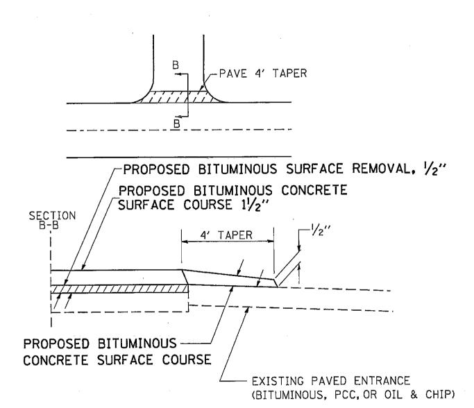
PREPARATION OF EXISTING SURFACE AND ANY EXCAVATION FOR ENTRANCES SHALL BE IN ACCORDANCE WITH ARTICLE 406.09 OF THE STANDARD OF SPECIFICATIONS.
