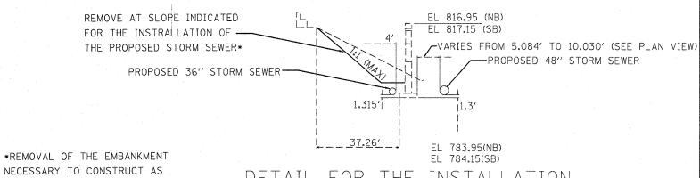
DETAIL FOR THE INSTALLATION OF PROPOSED STORM SEWER
