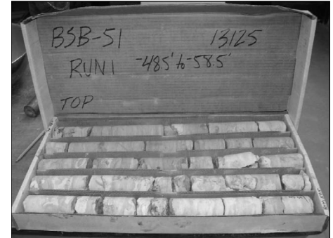
Color pictures of the cores Yes. Cores will be stored for examination for -- The "Strength" column represents the uniaxial compressive strength of the core sample (ASTM D-2938)
