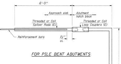
Bar Splicer for #5 bar Min. Capacity = 23.0 kips - tension Min. Pull-out Strength = 9.2 kips - tension No. Required =
